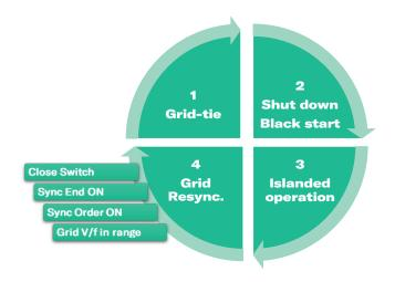
In addition, microgrids will also need to reconnect to the grid again and synchronize with the external grid.
