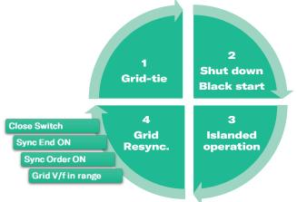
In addition, microgrids will also need to reconnect to the grid again and synchronize with the external grid.
